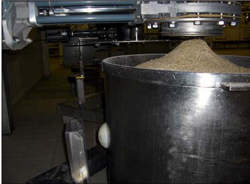
Lebkuchen Schmidt is using tagged mixing kettles to make sure each batch of baked goods has the correct ingredients, in the proper amounts.
